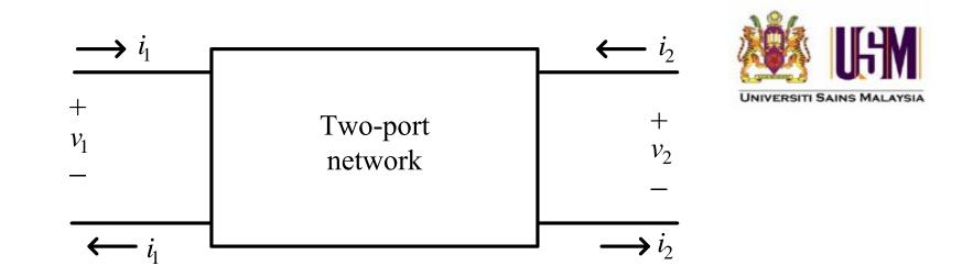
The model of an amplifier : one port represents the amplifier input characteristics and the other represents the output.
